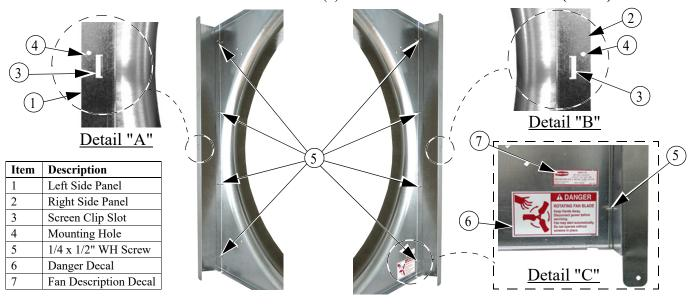
The Bottom Housing Panel has two Slots in it, and a full length bend (See Detail "A" below). The Flanges on the Bottom Housing Panel should overlap the Side Housing Panels (Detail "B"). Attach the Bottom Housing Panel to the bottom of the Shroud (the one with the Danger Decal) using the pre-drilled holes with four 1/4 x 1/2" Washer Head Screws. Attach the Bottom Housing Panel to the Side Panels
