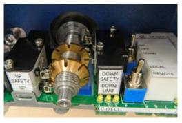
Toggle-style switches inside the unit permit the user to select local or remote operation. In local mode, the user can operate the unit manually while standing at the winch. This is particularly convenient for setting limit switches during installation and for making other adjustments.
